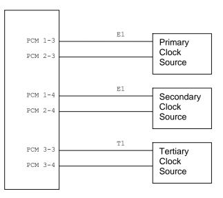
Figure 5 demonstrates a Signaling Gateway configured with three boards and six PCMs, four E1 and two T1 connect to primary, secondary and tertiary clock sources. Example MML for the above configuration is:
